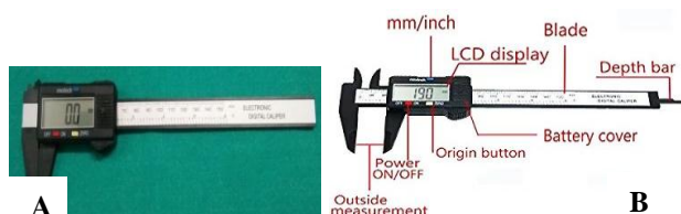
Figure 1 (A and B): Electronic digital caliper used in this study and its schematic representation.
